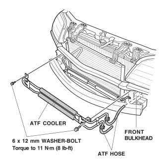
13. Remove the ATF return hose from the transmission, and from the radiator transmission cooler. Set the existing hose aside; it will not be reused. Attach the short ATF hose (return hose) from the new cooler to the radiator return hose fitting and secure them with an existing hose clamp.
