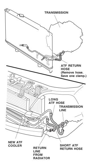
Attach the long ATF hose to the transmission line where you removed the return hose using one new hose clamp.  Attach the hose spacer between the two ATF hoses.
