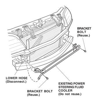
Attach the lower hose to the new power steering fluid cooler, and fit the cooler into position on the front bulkhead. Reinstall the two bracket bolts, and torque the bolts to 11 N·m (8 lb-ft).
