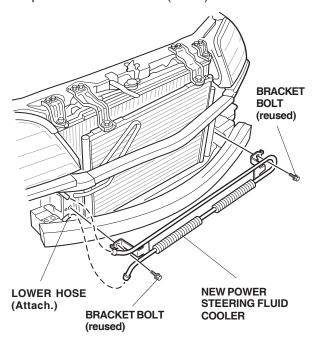
Reinstall the upper hose. Make sure that the hose is pushed firmly against the stopper on the cooler and that the dot on the upper hose is facing forward. Tighten the upper hose clamp to the specification shown.
