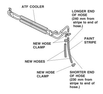
12. Route the hoses installed on the ATF cooler through the bulkhead, and fit the ATF cooler into position on the front bulkhead. Install the two 6 x 12 mm washer-bolts from the kit through the ATF cooler and into the threaded holes in the front bulkhead. Torque the bolts to 11 N·m (8 lb-ft).
